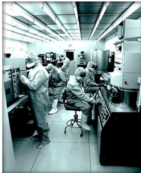
ITT gallium arsenide chip manufacturing process, which represents a "modern" Class 10 cleanroom system
