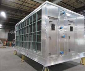
AC Corporation offers rental units, as well as complete and durable industrial custom-built air handling units designed to meet specific customer requirements. All units are fabricated and assembled in our factory and constructed on a rigid structural frame.
