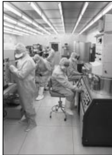
ITT gallium arsenide chip manufacturing process, which represents a "modern" Class 10 cleanroom system
